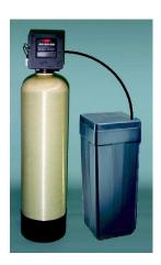
Akiki Engineering Filtration Series Commercial Softeners constructed based on efficient and economical method for removing feedwater hardness. Fiberglass vessels provide maximum corrosion-resistance and have a five-year warranty. Motor driven brass or Noryl control valves are easily programmed to adapt to specific system requirements. Polyethylene brine tanks, complete with support bed, are durable and corrosion resistant.
